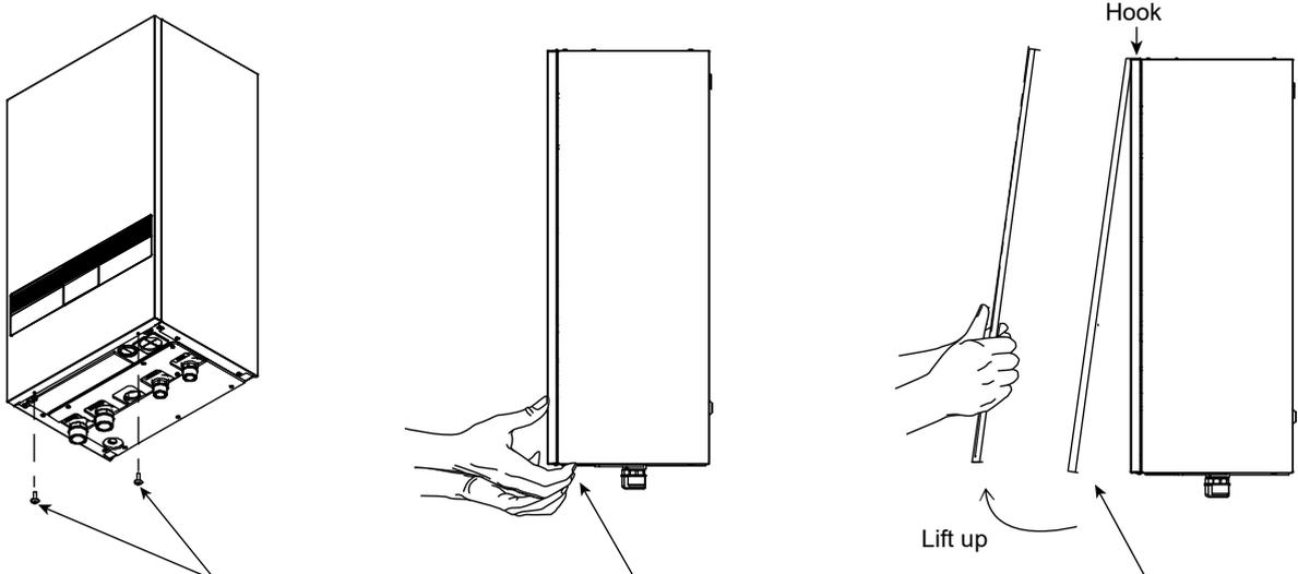
1. Remove the 2 mounting screws which located at bottom of the front plate.
