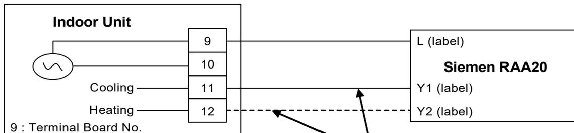
Connect only heating line for heating only model. And connect both heating and cooling line for heat + cool model.
