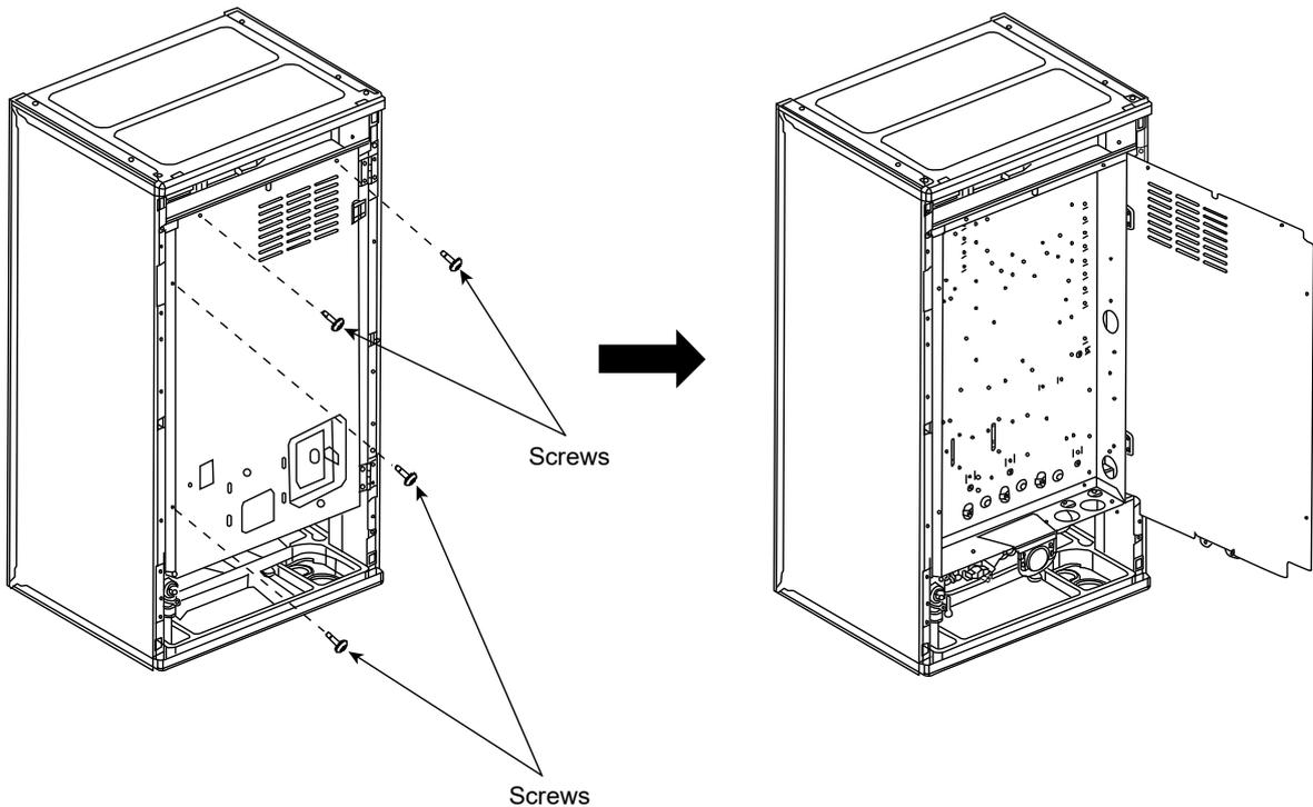
1. Remove 4 screws from the Control Board Cover.
