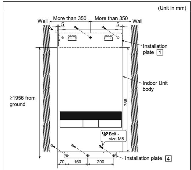
The centre of installation plate should be at more than 350 mm at right and left of the wall.
