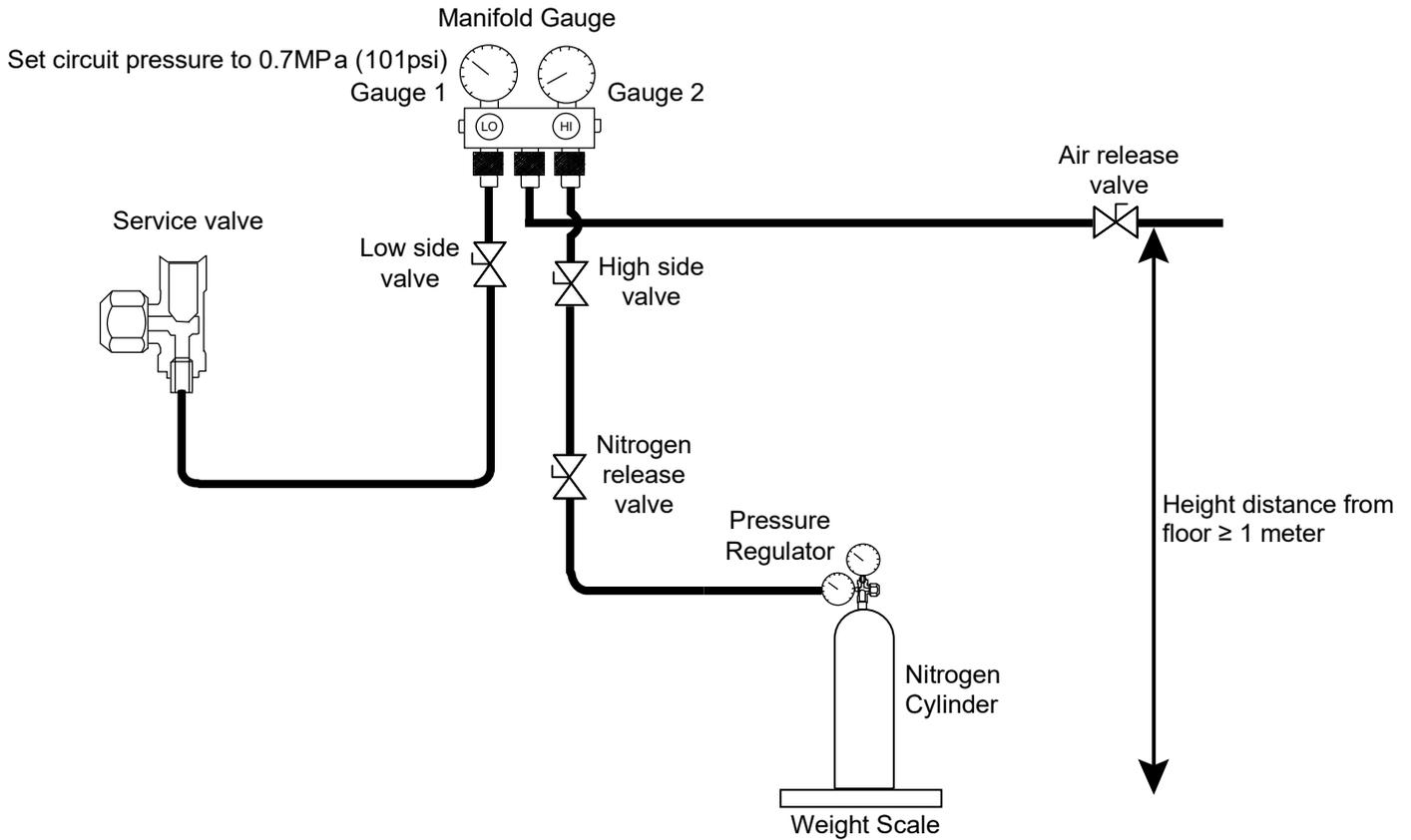
1. Connect nitrogen cylinder to the high side at the manifold gauge. Ensure nitrogen cylinder is connected to pressure regulator.
