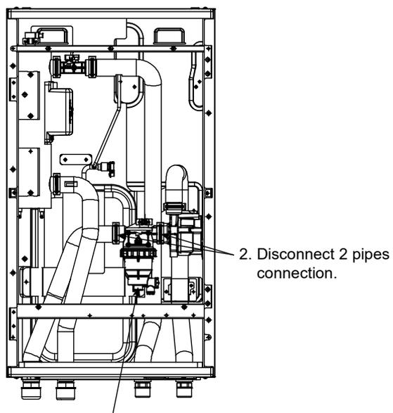
1. Turn to remove the Magnet Bar at bottom of Magnetic Water Filter Set.
