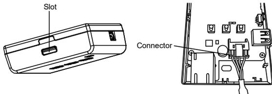
3. Pull the CN-CNT cable through the hole in the bottom of the adaptor and re-attach the front cover to the back cover.
