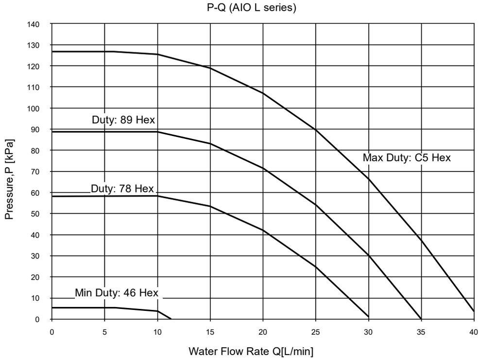
※ This condition is under connecting ODU and connecting 5m piping (inner diameter  $\Phi 25$ ) between ODU and IDU (AIO).
