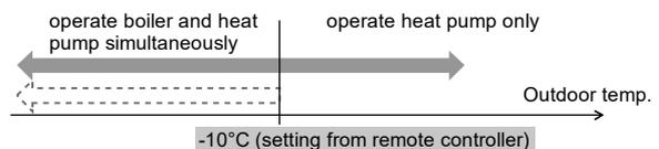
Although heat pump operates but water temperature does not reach this temperature for more than 30 mins (setting from remote controller)
