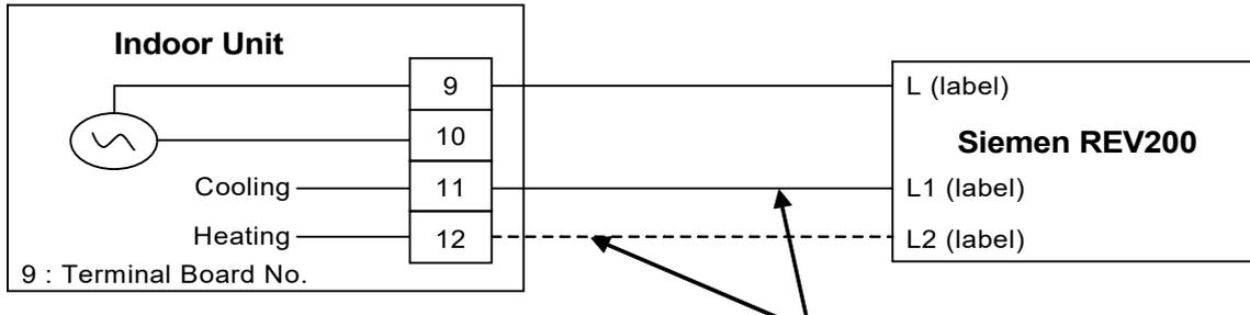
Connect only heating line for heating only model. And connect both heating and cooling line for heat + cool model.
