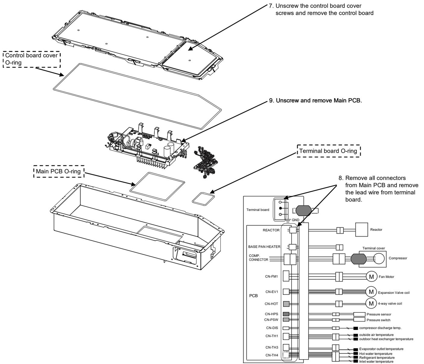
**Note:** During re-assemble the Main PCB, ensure to attach the O-ring properly to avoid gas leakage into the control board complete.
