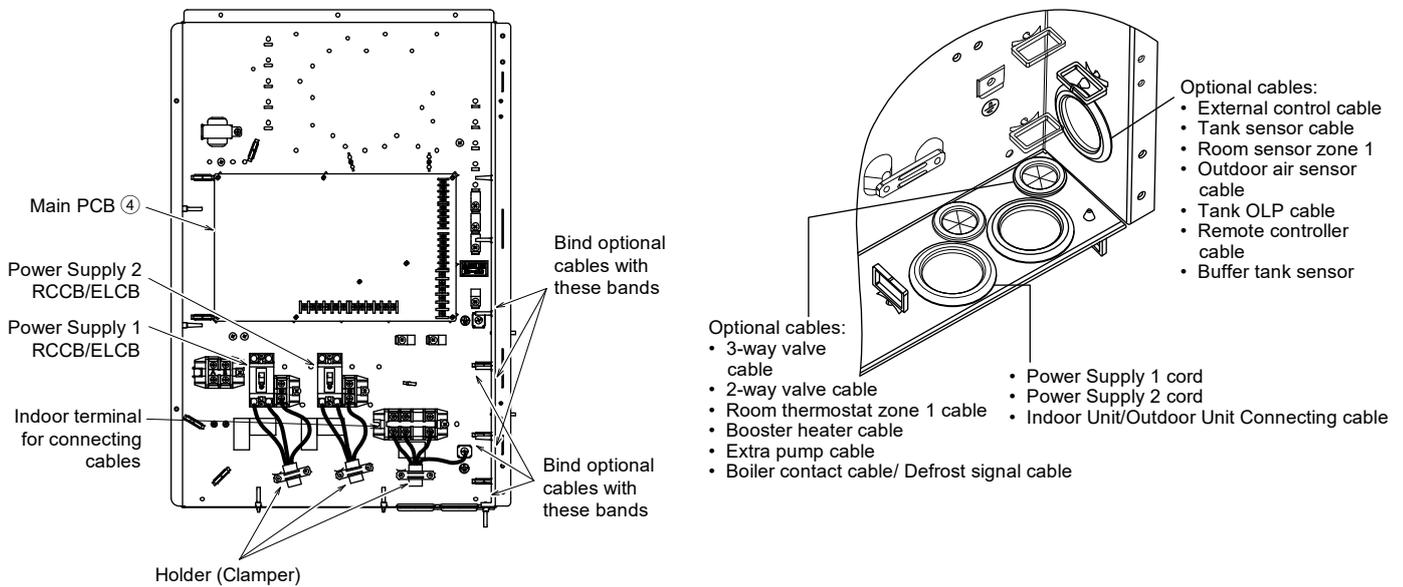
How to guide the optional cables and power supply cord
