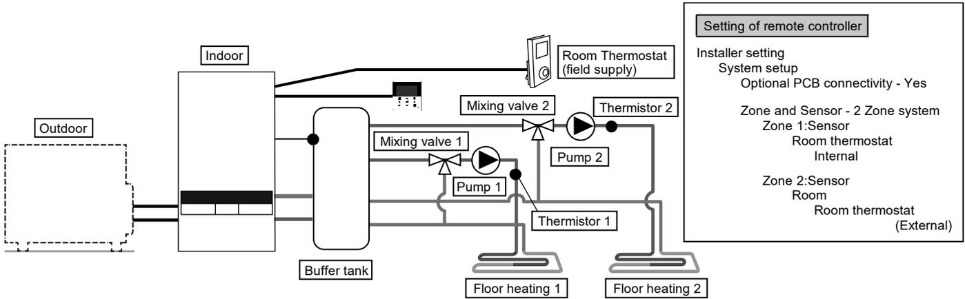
Connect floor heating to 2 circuits through buffer tank as shown in the figure.
