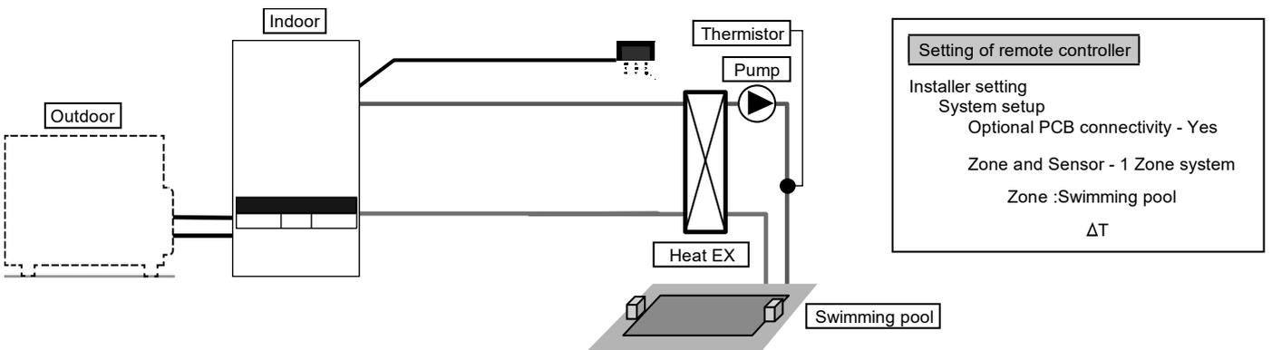
This is an application that connects to the swimming pool only. Connects pool heat exchanger directly to Indoor Unit without using buffer tank. Install pool pump and pool sensor (specified by Panasonic) at secondary side of the pool heat exchanger. Remove remote controller from Indoor Unit and install in room. Temperature of swimming pool can be set independently. This system requires the Optional PCB (CZ-NS5P).
