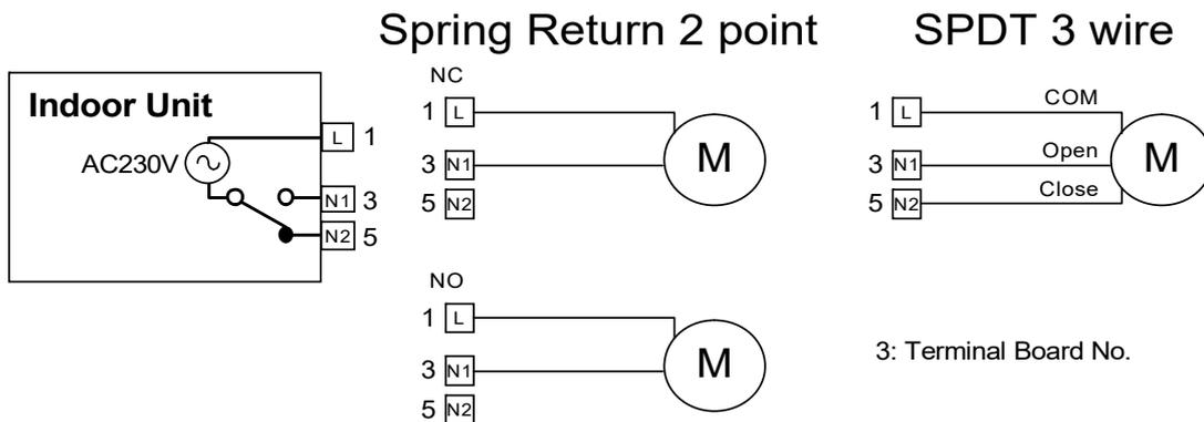
\* During pump down mode, fix 2 ways valve in close condition.
