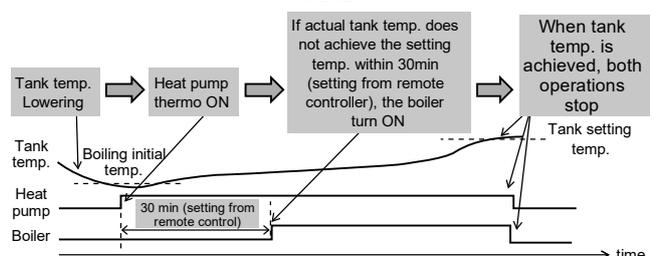
In Advanced Parallel mode, setting for both heating and tank can be made simultaneously. During operation of "Heating/Tank" mode, when each time the mode is switched, the boiler output will be reset to OFF. Please have good understanding on the boiler control characteristic in order to select the optimal setting for the system.
