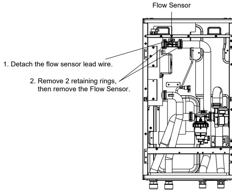
⚠ When reinstall Flow Switch, ensure the arrow on the flow switch is parallel with the pipe shaft and is facing in the direction of flow.
