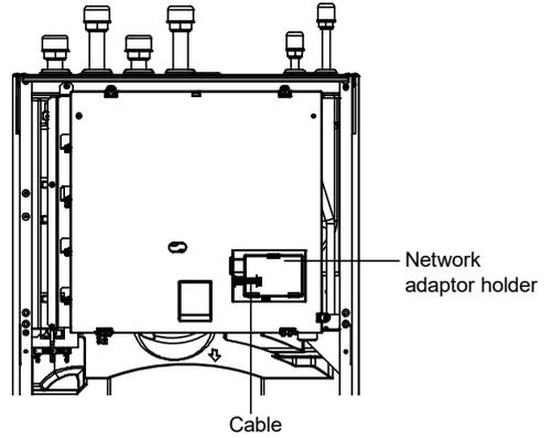
2. Connect cable coming out from the left side of the network adaptor holder to the connector inside the adaptor.
