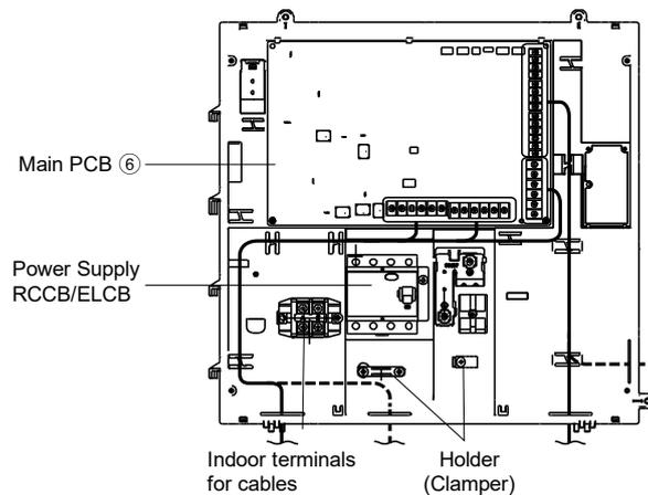
How to guide the optional cables and power supply cord connecting (view without internal wiring)
