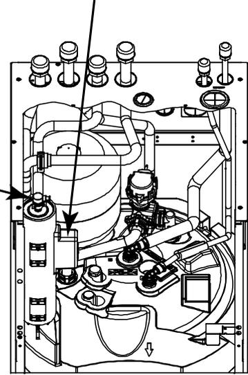
4. Disconnect 2 pipes connection and remove the bottle complete.
