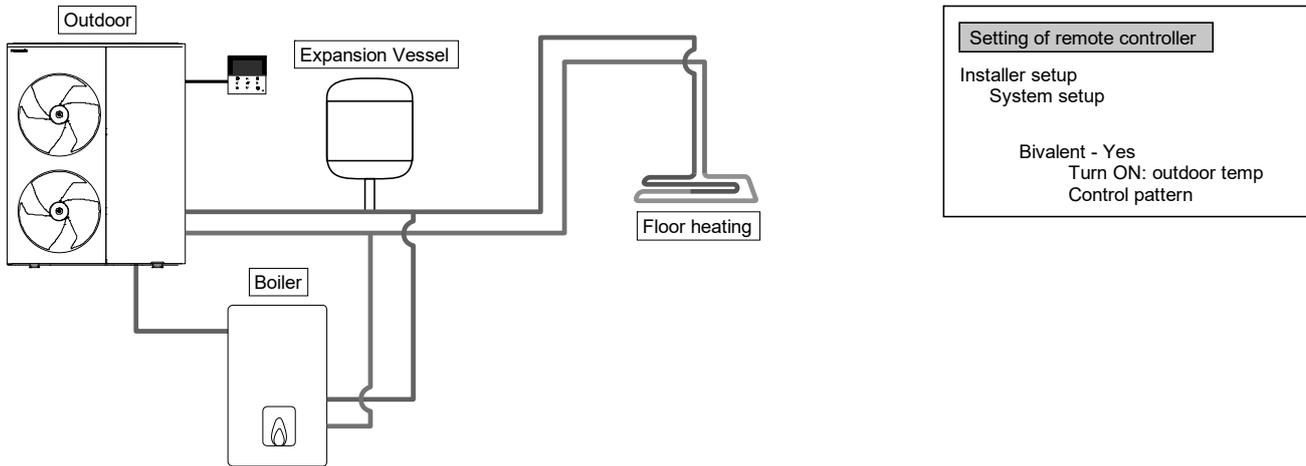
This is an application that connects the boiler to the Outdoor Unit, to compensate for insufficient capacity by operate boiler when outdoor temperature drops & heat pump capacity is insufficient.
