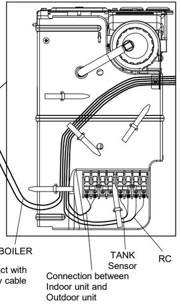
Route the cables as shown in the diagram above.
