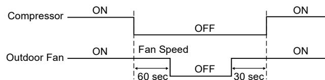
The reason the outdoor fan stops 60 seconds after the compressor stops is to exhaust heat.
