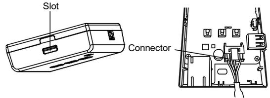
3. Pull the CN-CNT cable through the hole in the bottom of the adaptor and re-attach the front cover to the back cover.
