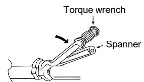
Refer to the table below for tightening torques for the water inlet and outlet.
