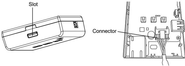
2. Pull the CN-CNT cable through the hole at the bottom of the adaptor and reattach the cover.
