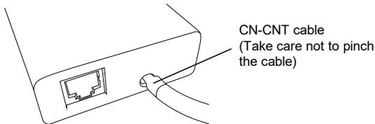
3. Connect the CN-CNT cable to the CN-CNT connector on the outdoor unit.
