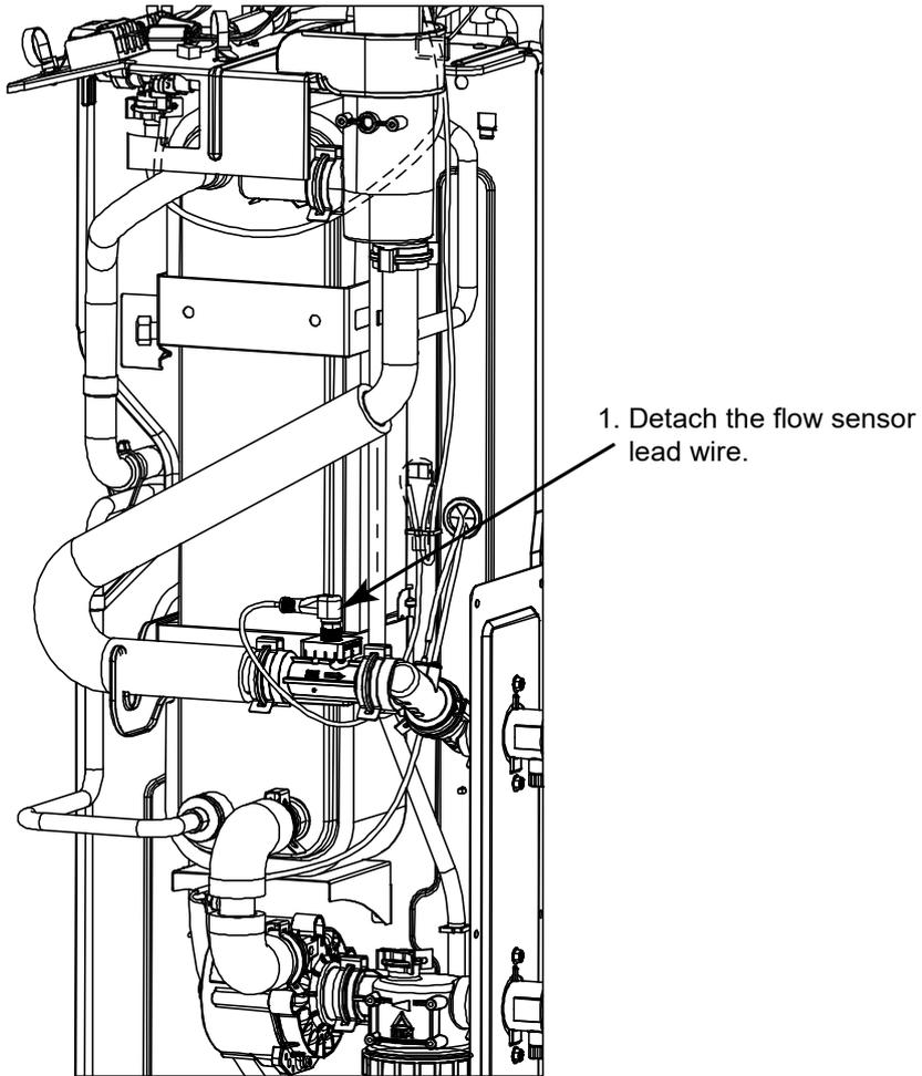
⚠ When reinstall Flow sensor, ensure the arrow on the flow sensor is parallel with the pipe shaft and is facing in the direction of flow.
