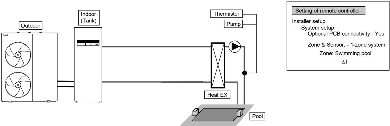
This is an application that connect to the swimming pool only. Connect the pool heat exchanger directly to the tank unit without using buffer tank. Install a pool pump and pool thermistor (specified by Panasonic) at the secondary side of the pool heat exchanger. The pool temperature can be set with a remote controller. This system requires the Optional PCB (CZ-NS6P). The cooling mode cannot be selected for this application. (Not displayed on the remote controller).
