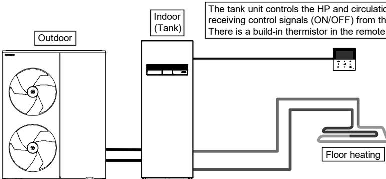
The tank unit controls the HP and circulation pumps by receiving control signals (ON/OFF) from the remote controller. There is a build-in thermistor in the remote controller.
