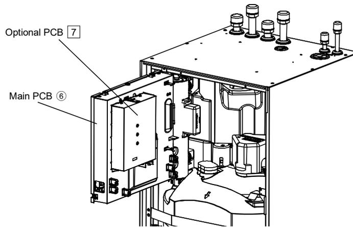
\* For installation on how to route lead wires between Optional PCB 7 and main PCB 6, please refer to the "Optional PCB (CZ-NS6P)" manual.
