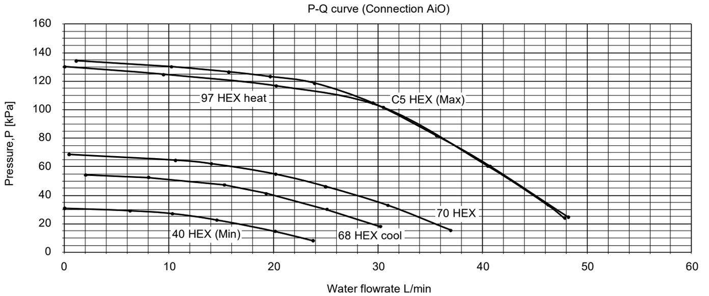
※ This condition is under connecting ODU and connecting 5m piping (inner diameter  $\Phi 25$ ) between ODU and IDU (AiO).
