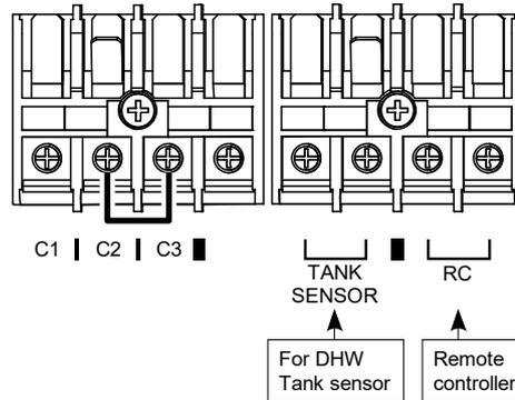
When connecting to an indoor unit, remove the short-circuit wires "C2" and "C3" and connect as shown in the diagram below.
