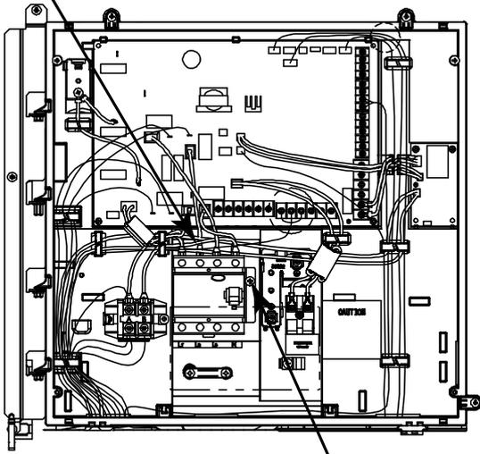
3. Remove screw and bracket to remove the RCCB.
