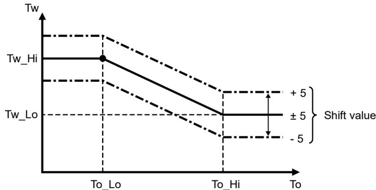
**14.1.5 Target Water Temperature at Extension System (Optional PCB is Connected, Excluding when Operating in Standalone)**
