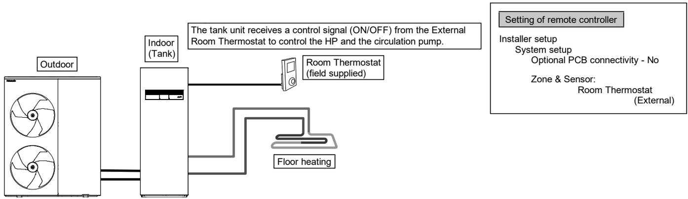
Connect floor heating and radiators directly to the tank unit.
