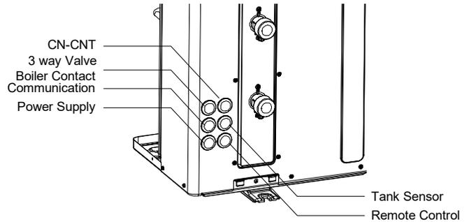
Pull the power supply cable and connecting cable through the Connecting Cable Hole ⑬ as shown in the illustration.
