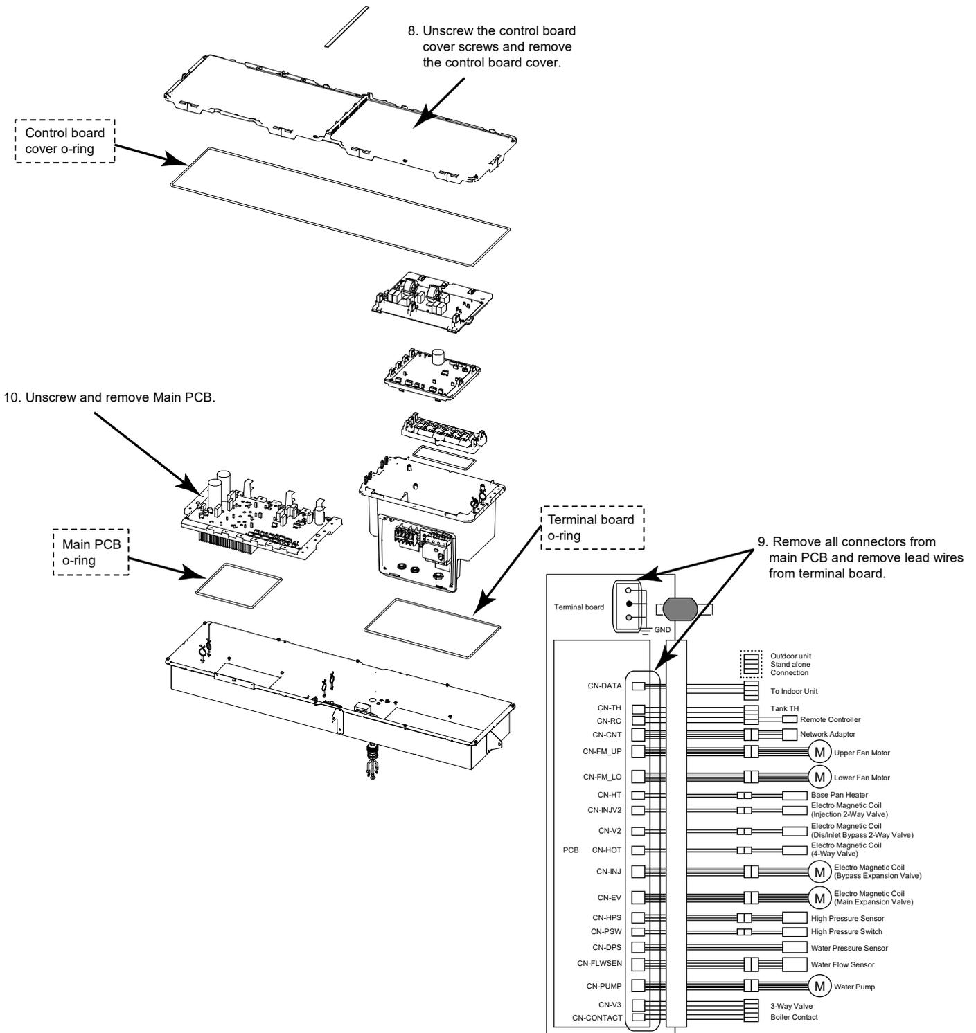
Note: During re-assemble the Main PCB, ensure to attach the O-ring properly to avoid gas leakage into the control board complete.
