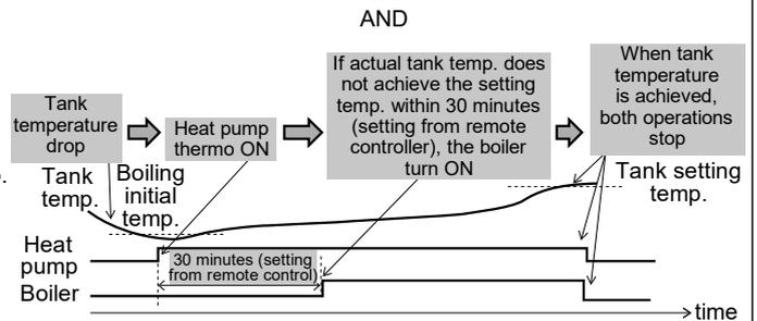
In Advanced Parallel mode, setting for both Heat and Tank can be made simultaneously. During operation of "Heat/Tank" mode, when each time the mode is switched, the boiler output will be reset to OFF. Please have good understanding on the boiler control characteristic in order to select the optimal setting for the system.
