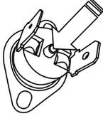
Press this button with a test pen to reset (10).
