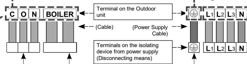
Need to connect when using an optional DHW tank
