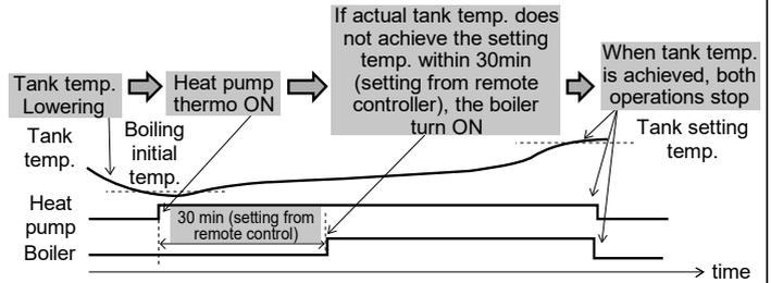
In Advanced Parallel mode, setting for both heating and tank can be made simultaneously. During operation of "Heating/Tank" mode, when each time the mode is switched, the boiler output will be reset to OFF. Please have good understanding on the boiler control characteristic in order to select the optimal setting for the system.
